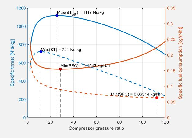
Calculation of the both engines engine was prowided for the same TIT (Tt4) and for the same flight codition (H, M0). For AB ON mode aditionaly TAB was specified
