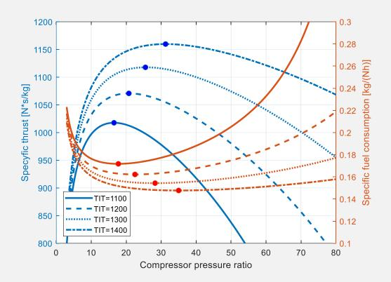
SFC is lower for higher TIT (it is slightly different than for turbojet without AB) The difference between CPRs for max ST and min SFC grows for higher TIT
