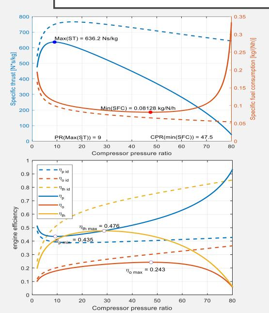
Calculation of the real and the ideal engine was prowided for the same TIT ( $T_{t4}$ ) and for the same flight codition (H, M<sub>0</sub>)
