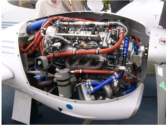
Diamond DA42 Twin Star Thielert Centurion 1.7 diesel engine
